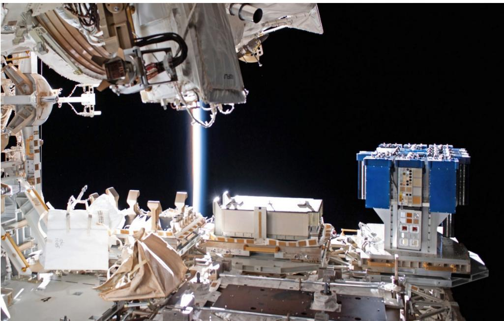
*Figure 11. The wake side of the MISSE-FF with the MISSE-10 PCE-2 and MISSE-12 PCE-3 MSCs as photographed on January 25, 2020 during an EVA. The MSCs are closed, except for the central wake MSC which is open (iss061e143021).*
