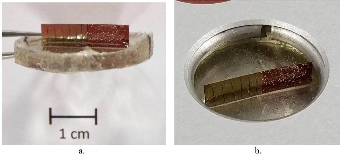
Figure 21. Pre-flight photographs of the PCE-2 sample Au-Kapton H/Ni (M10Z-C4): a). As fabricated, and b). As mounted in the M10 Z2 MSC 10 MS deck.
