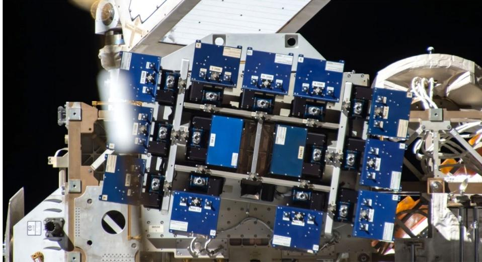
*Figure 9. An on-orbit image taken on January 16, 2019 showing the top of the MISSE-FF with the MISSE-9 and MISSE-10 MSCs installed (iss058e003972).*
