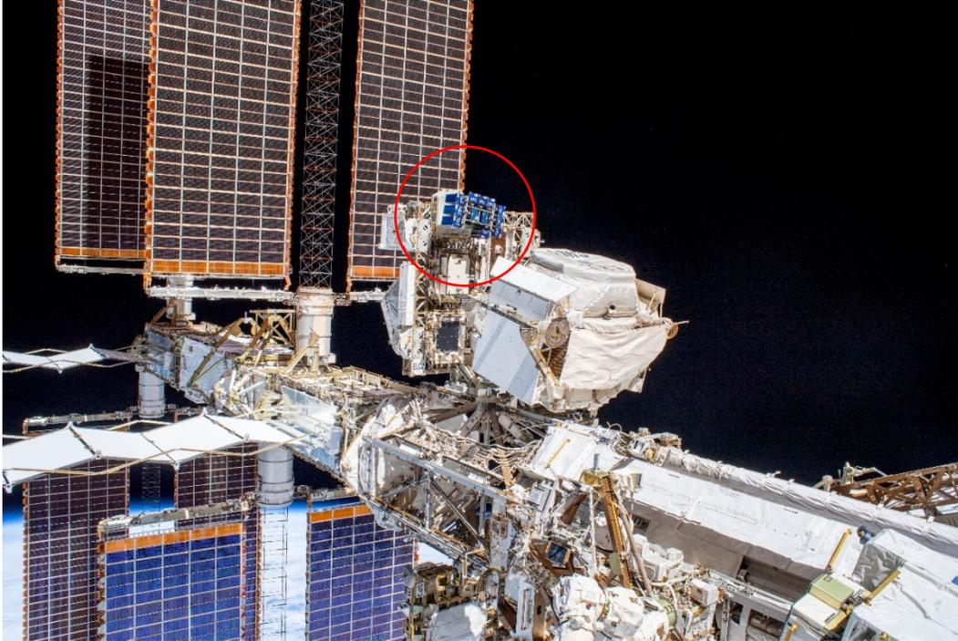
*Figure 8. A view of the MISSE-FF on ELC-2 Site 3 as photographed during an EVA on November 15, 2019 (iss061e040917).*
