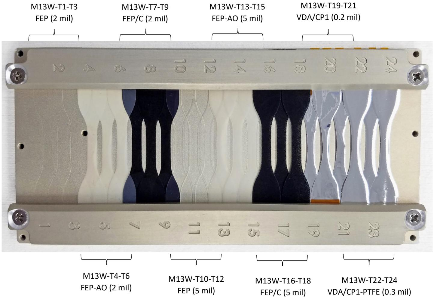
Figure A-14. MISSE-13 PCE-4 wake tensile samples. All samples are cut parallel to the roll direction (PtR).
