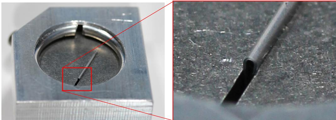
*Figure 38. Pre-flight photograph of aluminized-Teflon FEP under folding stress (M13W-C5).*
