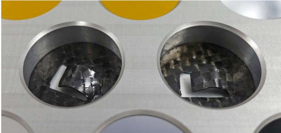
Figure 31. Pre-flight photograph of the MISSE-12 ram SMC samples in the R2 MSC 4 SS deck (M12R-C27 (left) and M12R-C28 (right)).
