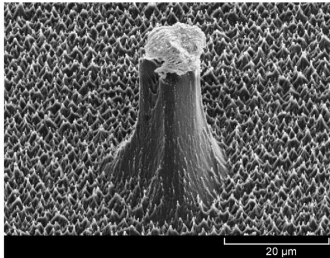
Figure 1. Atomic oxygen erosion of Teflon FEP after 5.8 years of space exposure.<sup>2,7</sup>
