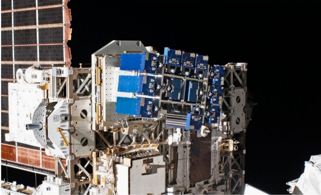
*Figure 10. Close-up image of the MISSE-FF with the MISSE-10 PCE-2 and MISSE-12 PCE-3 MSCs as photographed during an EVA on January 25, 2020. The front surface of the blue ram MSCs can be seen in the closed position (iss061e142772).*
