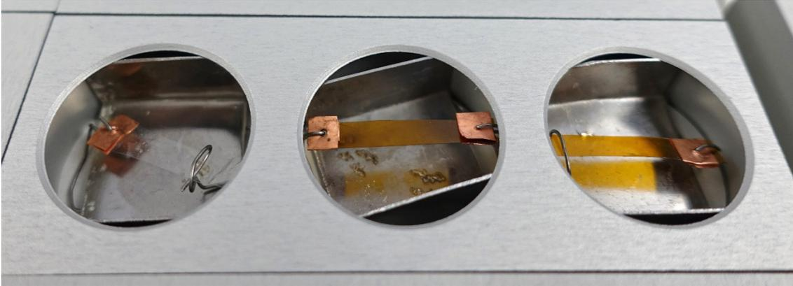
Figure 30. Close-up photograph of 3 tensile loaded MISSE-12 samples in the W3 MSC 6 MS deck (M12W-C18 (left), M12W-C17 (center), M12W-C16 (right)).
