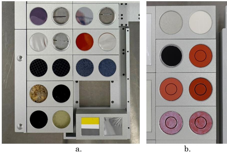
Figure 42. Close-up photographs of the MISSE-13 PCE-4 samples loaded into the MSC flight decks: a). Lower section of samples in W1 MSC 19 MS (wake), b). Upper section of samples in W1 MSC 19 MS (wake), c). Samples in W1 MSC 19 SS (wake), and c). Samples in Z2 MSC 5 MS (zenith).
