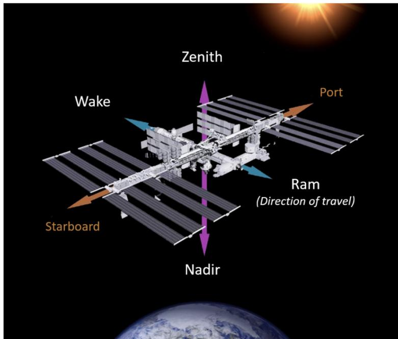
*Figure 7. Diagram showing ram, wake, zenith, and nadir directions on the International Space Station.*
