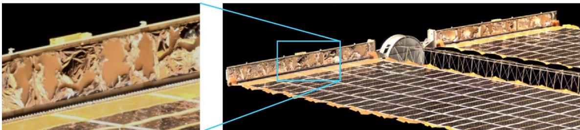
Figure 3. Atomic oxygen undercutting degradation of the P6 Truss solar array wing blanket box cover on the ISS after only 1 year of space exposure.<sup>10</sup>
