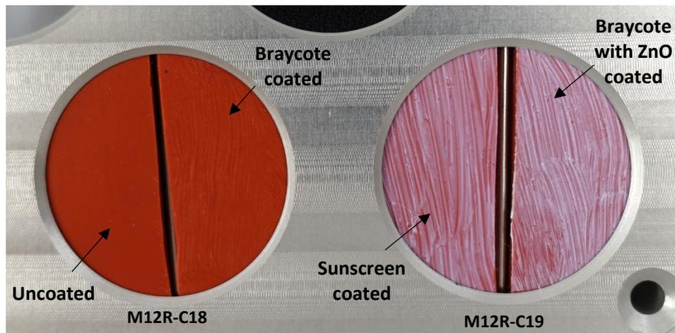
Figure 29. Pre-flight photograph of the MISSE-12 ram coated and uncoated docking seal material samples M12R-C18 (left) and M12R-C19 (right).
