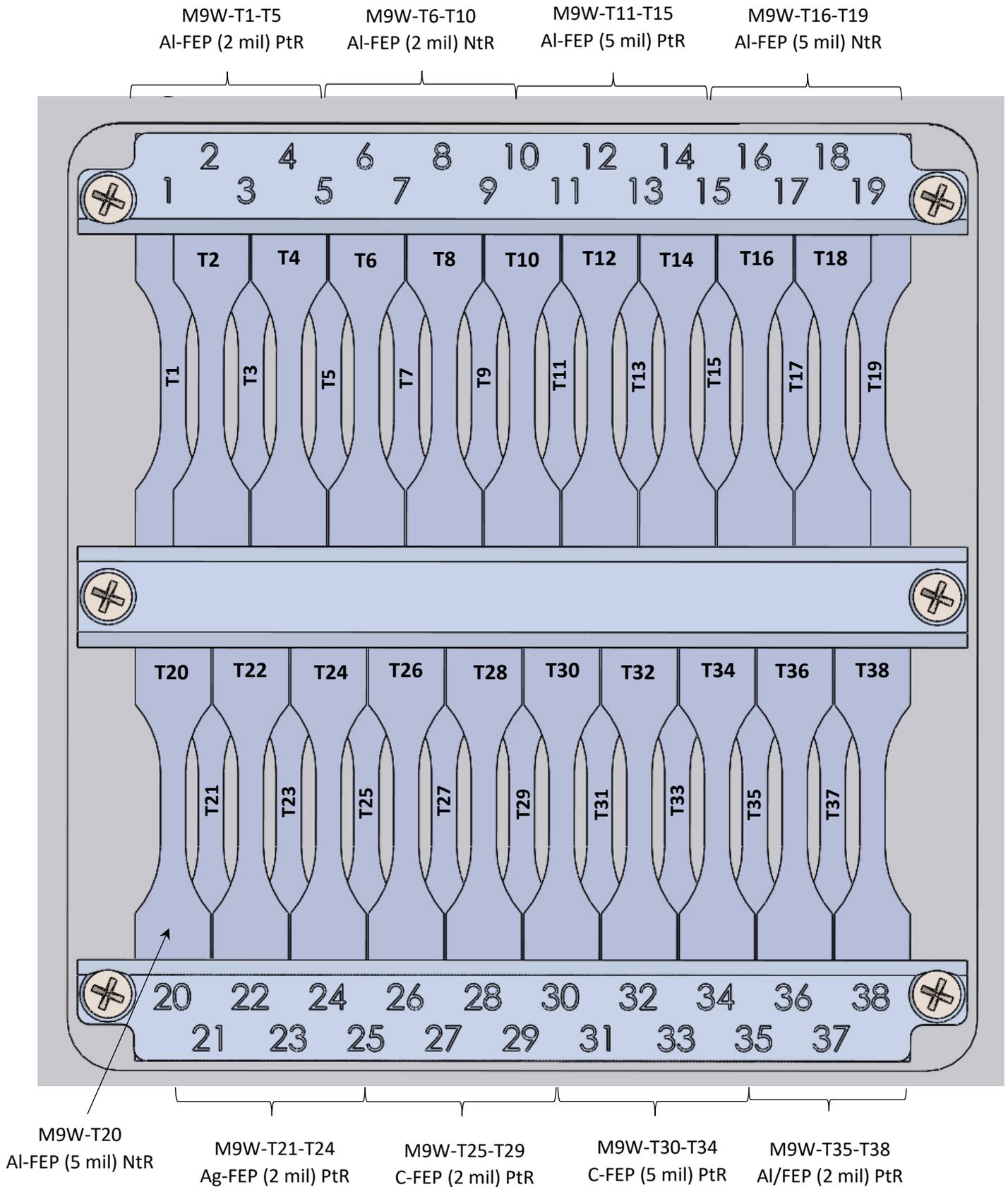
Figure A-3. MISSE-9 PCE-1 wake tensile samples. Samples cut parallel to the roll direction are designated as PtR and samples cut normal to the roll direction are designated as NtR.
