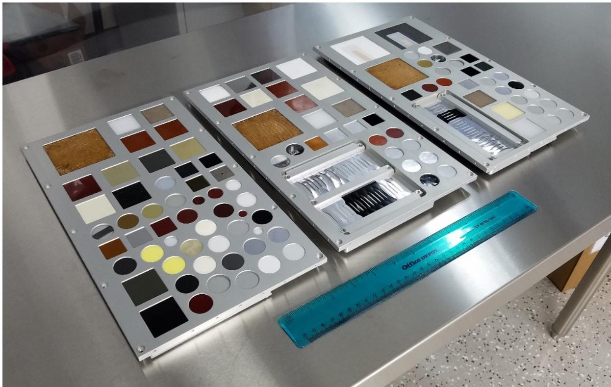
*Figure 15. Pre-flight photograph of the MISSE-9 PCE-1 samples loaded into the MSC MS flight decks, from left to right: R2 MSC 3 (ram), W3 MSC 8 (wake), and Z3 MSC 5 (zenith).*
