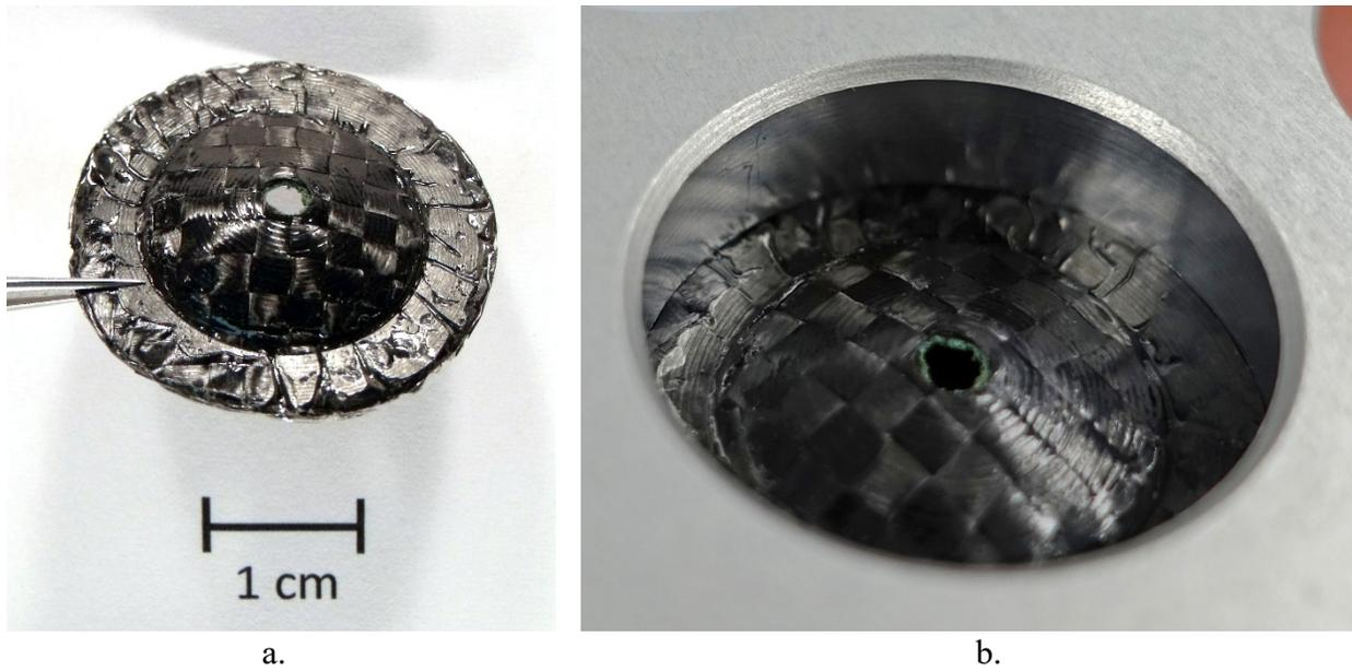
Figure 23. Pre-flight photographs of the nadir SMC sample (M10N-C9): a). Prior to integration showing the dome shape, and b). Integrated in the N3 MSC 13 MS deck with an aluminum spacer at the outer circumference.
