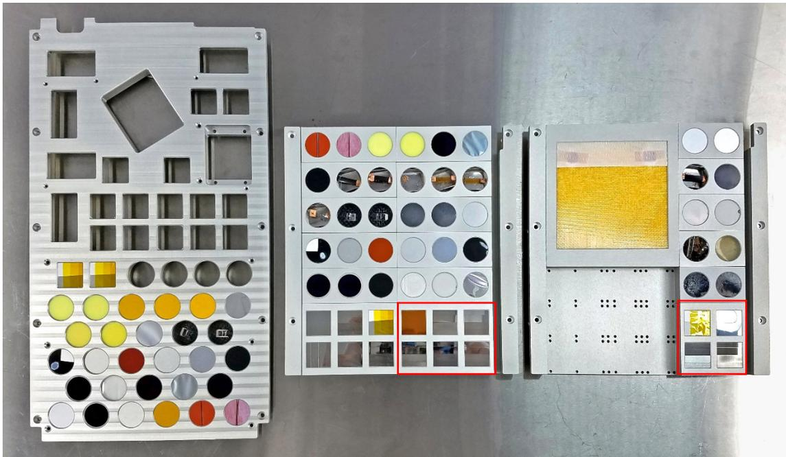
*Figure 33. Pre-flight photograph of the MISSE-12 PCE-3 samples loaded into the MSC flight decks, from left to right: R2 MSC 4 SS (ram), W3 MSC 6 MS (wake) and Z1 MSC 18 MS (zenith). The large yellow sample in Z1 MSC 18 MS is not part of the PCE-3. Samples in red boxes were moved to a different location on the deck prior to flight.*
