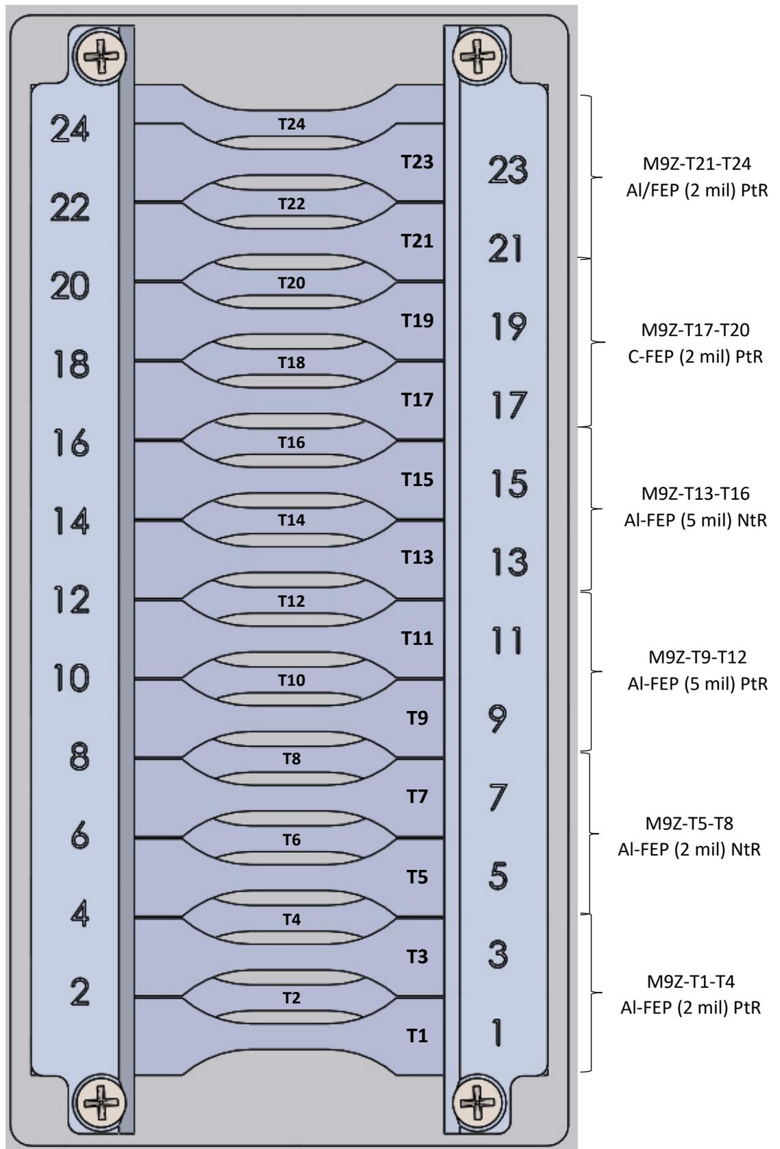
Figure A-5. MISSE-9 PCE-1 zenith tensile samples. Samples cut parallel to the roll direction are designated as PtR and samples cut normal to the roll direction are designated as NtR.
