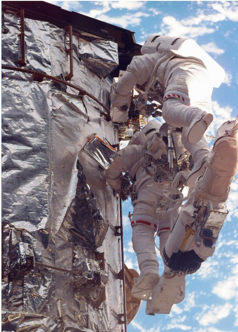
*Figure 4. Large cracks in the HST Light Shield solar facing MLI as observed during SM2, after 6.8 years in space.<sup>21</sup>*
