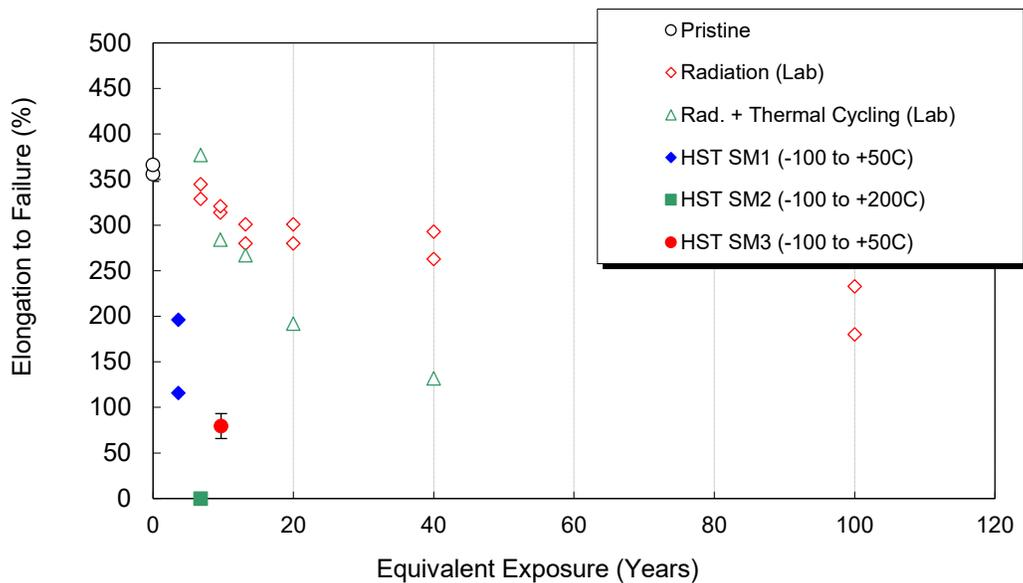
Figure 6. Ground laboratory data for radiation and thermal cycling exposure of 5 mil FEP simulating up to 100 mission years on HST.<sup>24,29</sup>
