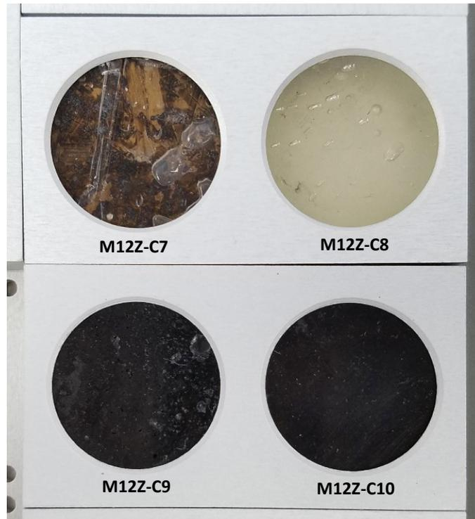
Figure 28. Pre-flight photograph of the melanin-based samples in the MISSE-12 Z1 MSC MS deck.
