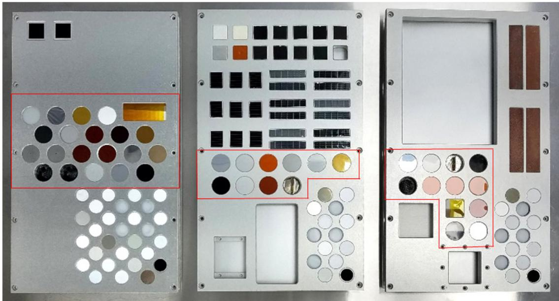
Figure 24. Pre-flight photograph of the MISSE-10 PCE-2 samples loaded into the MSC MS flight decks, from left to right: R1 MSC 11 (ram), Z2 MSC 10 (zenith), and N3 MSC 13 (wake). The PCE-2 samples are shown outlined in red.
