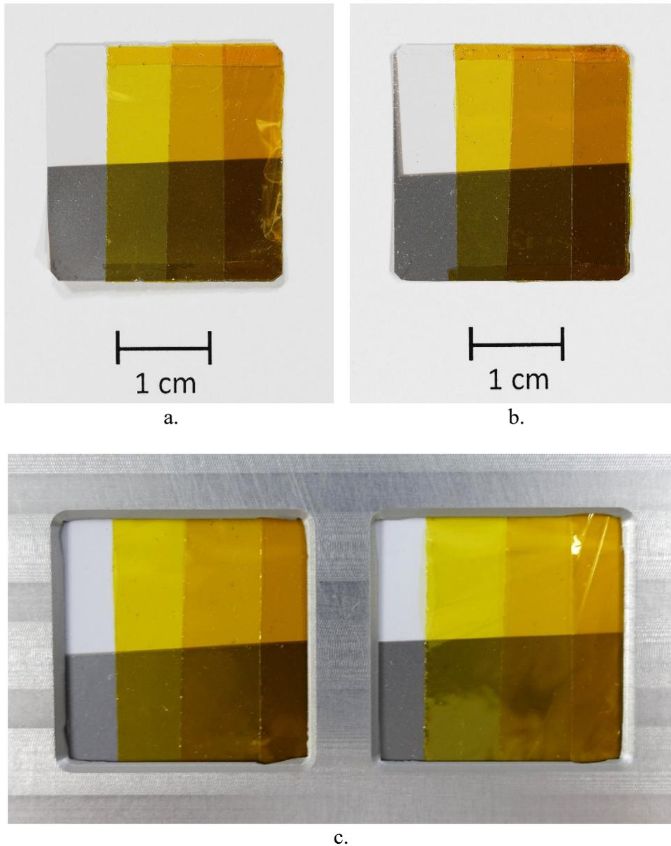
Figure 26. Pre-flight photographs of the PCE-3 Photographic AO Monitors: a). M12R-S1 with 0.3 mil Kapton H layers, b). M12R-S2 with 0.5 mil Kapton H layers, and c). M12R-S1 (right) and M12R-S2 (left) mounted in the M12 R2 SS deck.
