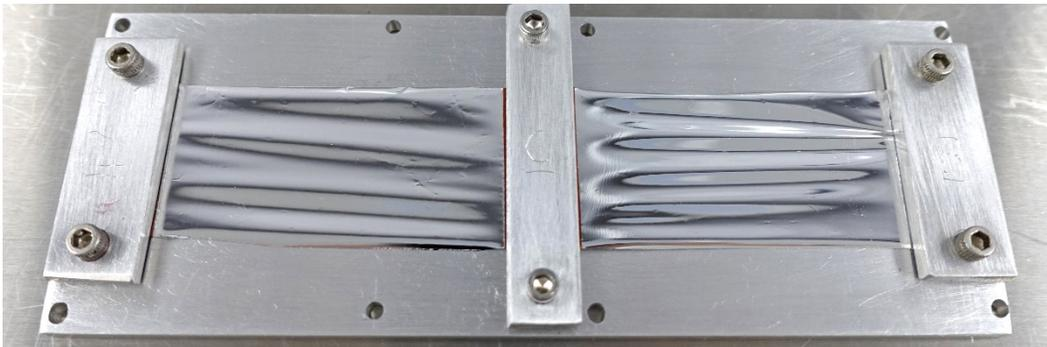
*Figure 37. Pre-flight photograph of the stretched solar sail samples mounted on the MISSE-13 W1 MSC 19 SS flight deck. Sample 13W-SR1 is on the right and sample M13W-SR2 is on the left.*
