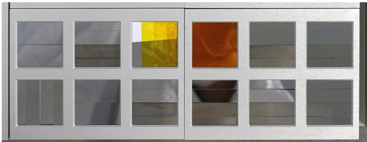
*Figure 27. Close-up pre-flight photograph of the MISSE-12 wake SMA samples.*
