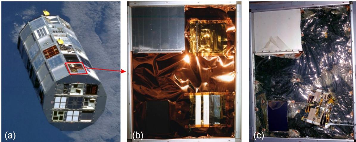
Figure 2. Atomic oxygen erosion of a Kapton insulation blanket from LDEF experiment Tray F-9, located on the leading edge and exposed to direct-ram AO for 5.8 years.<sup>7</sup>
