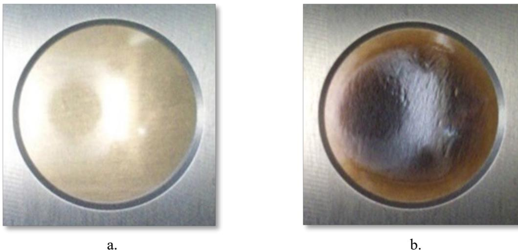
*Figure 18. On-orbit images of the PCE wake PVC sample (M9W-C8): (a). Image taken on April 23, 2018 shortly after deployment, and (b). Image taken on December 26, 2018 after 6.4 months of space exposure. (Photo credit: Alpha Space)*
