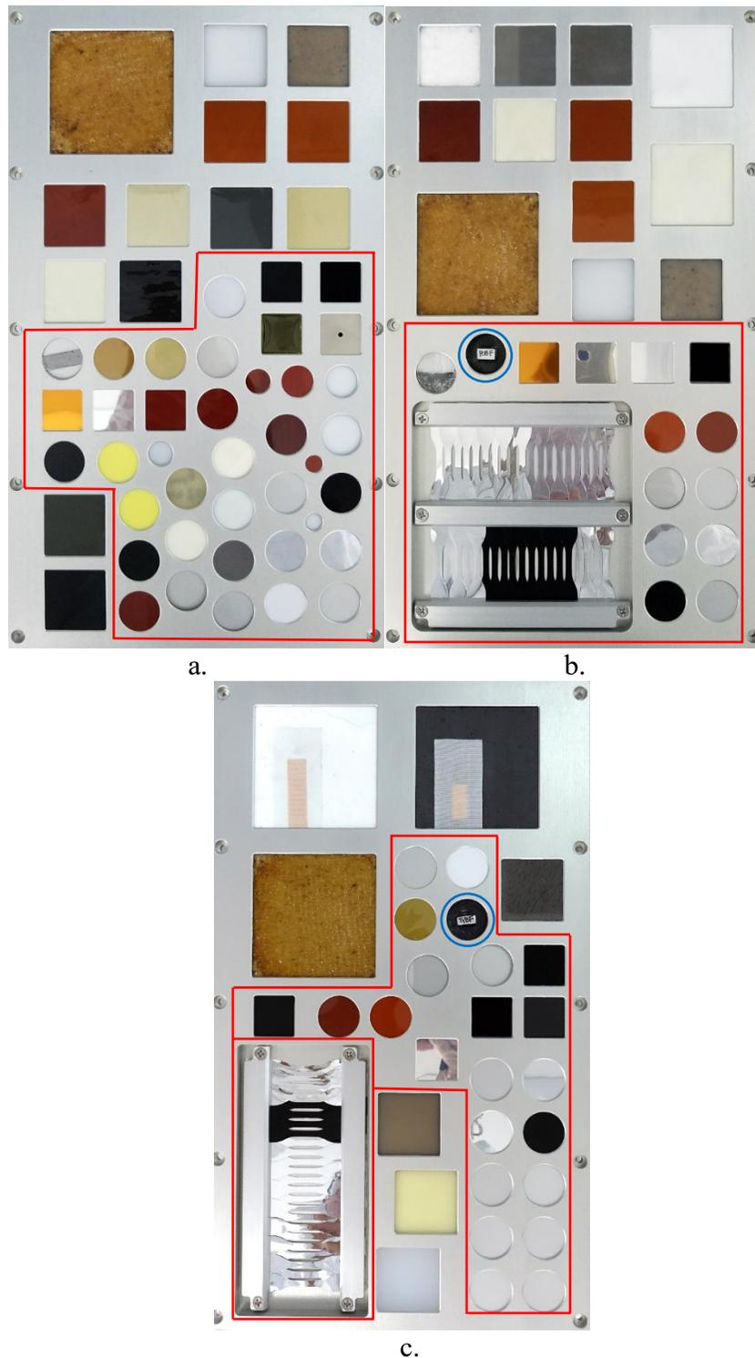
Figure 16. Pre-flight photographs of the MISSE-9 MSC decks with the PCE-1 samples outlined in red: a). Ram samples in the R2 MSC 3 MS deck, b). Wake samples in the W3MSC 8 MS deck (the sample with the “RBF” block is circled in blue), and c). Zenith samples in the Z3 MSC 5 MS deck (the sample with the “RBF” block is circled in blue).
