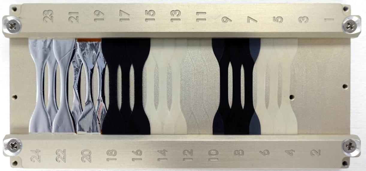
*Figure 36. Pre-flight photograph of the MISSE-13 wake tensile samples mounted in the MISSE-13 W1 MSC 19 SS tensile flight holder with sample ID bars.*
