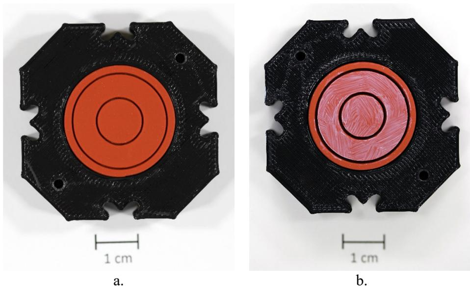
Figure 40. Pre-flight photographs of two of the PCE-4 zenith seal flight samples: a). Uncoated S0383-70 silicone seal (M13Z-C7), and b). S0383-70 silicone coated with Dow Corning 7 + ZnO (DCZ) sunscreen (M13Z-C10).
