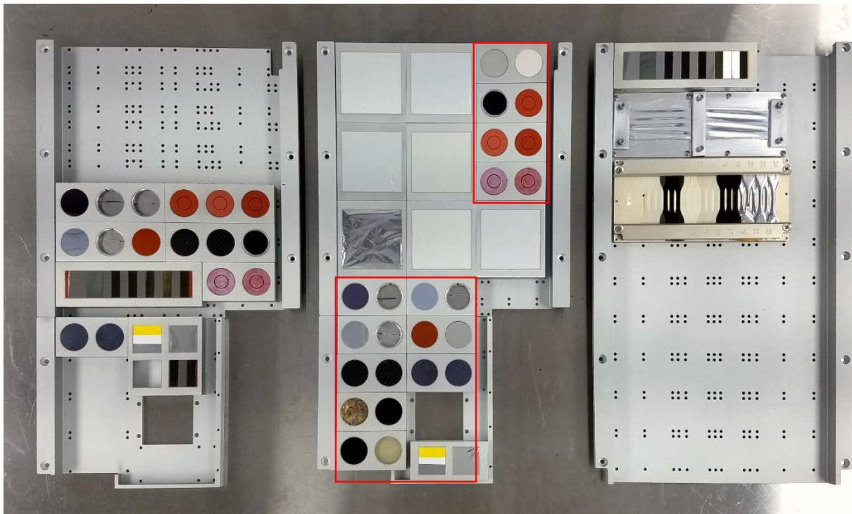
*Figure 41. Pre-flight photograph of the MISSE-13 PCE-4 samples loaded into the MSC flight decks, from left to right: Z2 MSC 19 MS (zenith), W1 MSC 19 MS (wake) and W1 MSC 19 SS (wake). The PCE-4 samples in the wake MS deck are outlined in red.*
