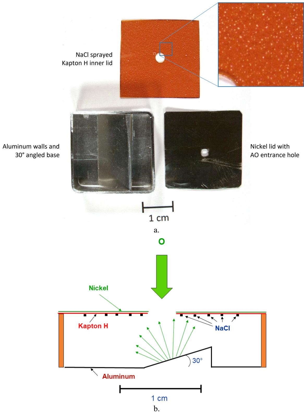
Figure 12. PCE-1 AO Scattering Chamber (M9R-S7): a). Pre-flight photograph of the individual components including a close-up image of the salt-sprayed Kapton inner lid, and b). Schematic diagram of the assembled AO Scattering Chamber.
