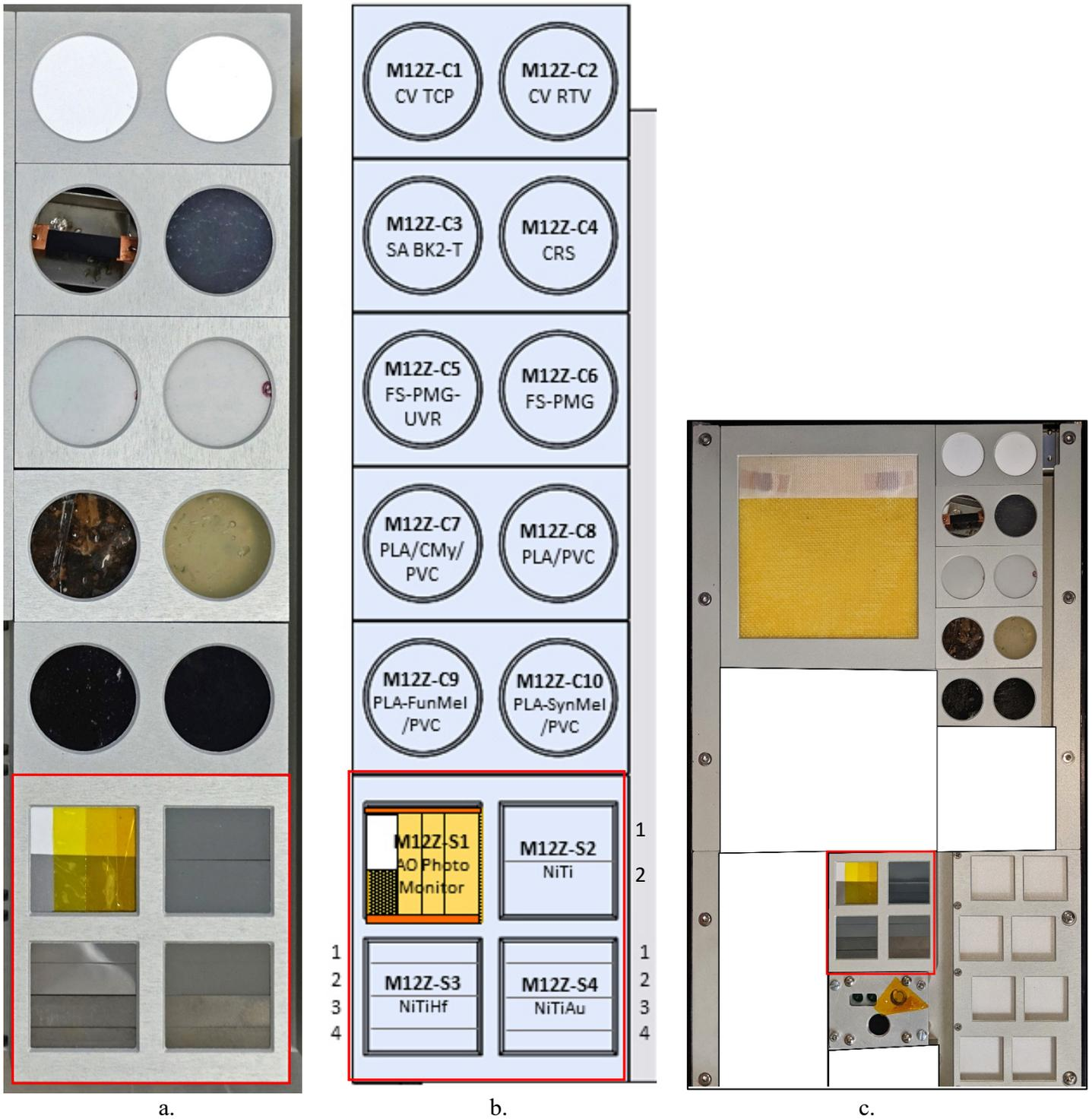
Figure A-11. MISSE-12 PCE-3 zenith samples: a). Pre-flight photo of the PCE-3 sample area of the M12 Z1 (MSC 18) MS deck prior to re-positioning the bottom 4 samples (outlined in red), b). The PCE-3 M12 Z1 sample map, and c). Pre-flight photo of the PCE-3 Z1 MS deck after re-positioning the 4 samples (Alpha Space photograph with other samples whited-out).
