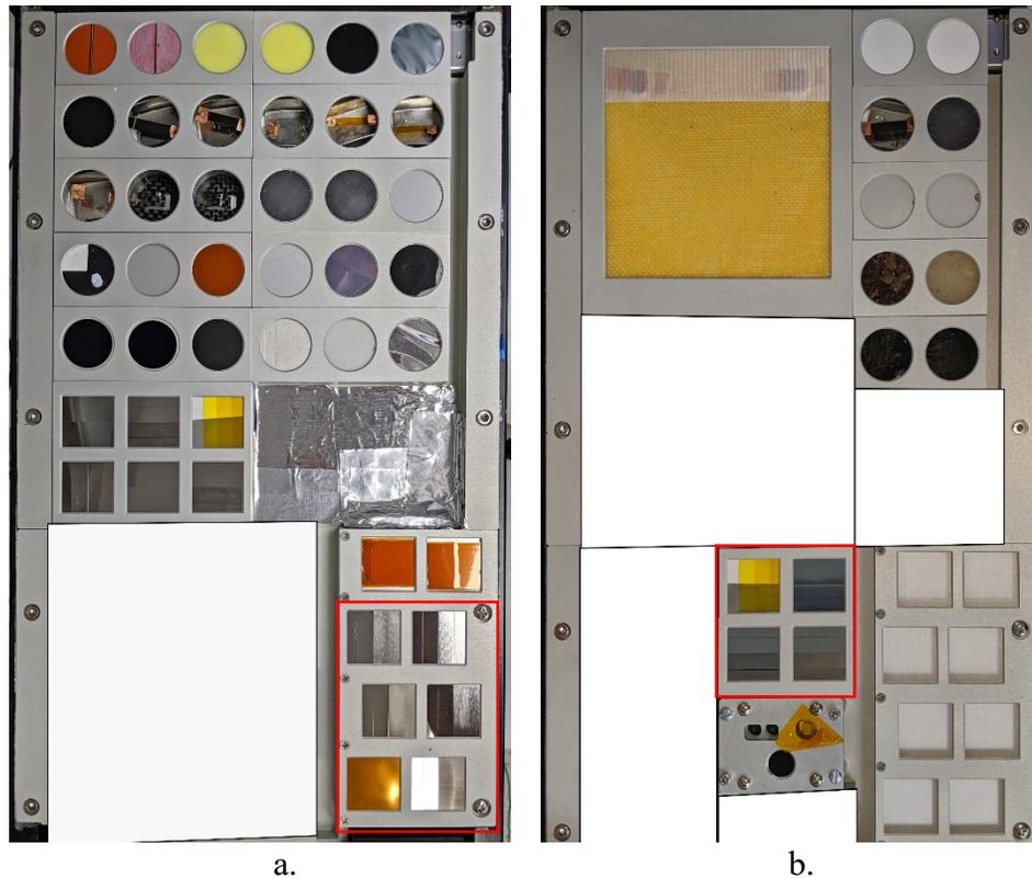
Figure 35. Final deck configuration of the MISSE-12 wake and zenith MSC flight decks: a). W3 MSC 6 MS (wake), and b). Z1 MSC 18 MS (zenith). The moved samples are in the red-box areas. (Photo credit: Alpha Space)
