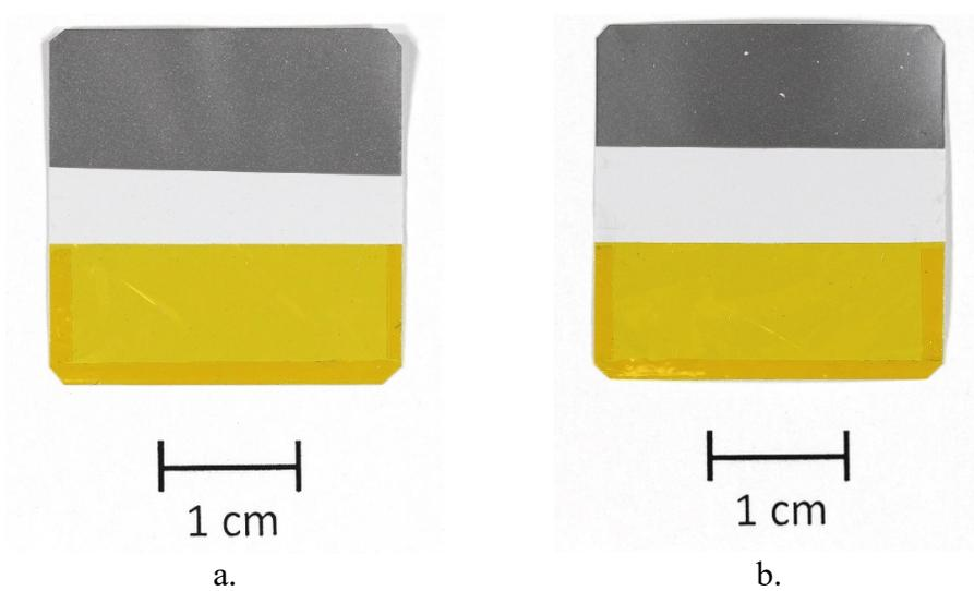
Figure 39. Pre-flight photographs of the PCE-4 AO Photographic Monitor flight samples: a). Wake monitor (M13W-S1), and b). Zenith monitor (M13Z-S1).
